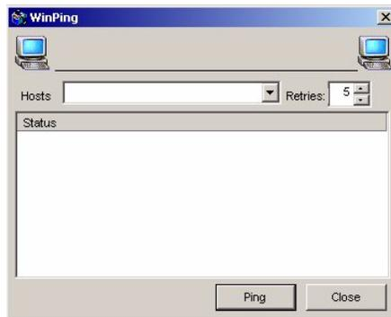
WinPing is a diagnostic tool that sends an echo request to a network host. The host parameter is either a valid host name or an IP address. If the host is operational and on the network, it responds to the echo request. The default is to send 5 echo requests and then stop if no response is detected. WinPing sends one echo request per second, calculates round trip times and packet loss statistics, and displays a brief summary upon completion.
