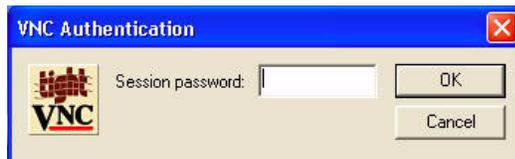
5. Enter the **Session password** of the thin client that is to be operated/monitored (this is the password used in the **WinVNC: Current User Properties** dialog box of the thin client) and click **OK**.
